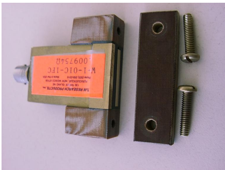
Picture 7: W shunt including accessories
