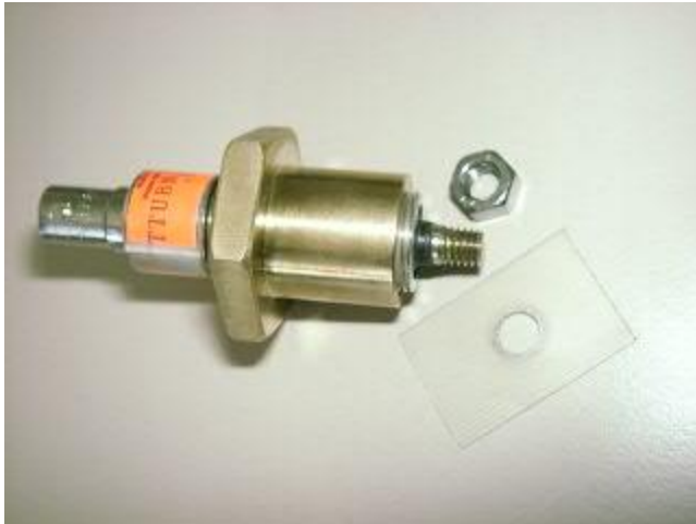
Picture 1: SBNC shunt with isolation plate
