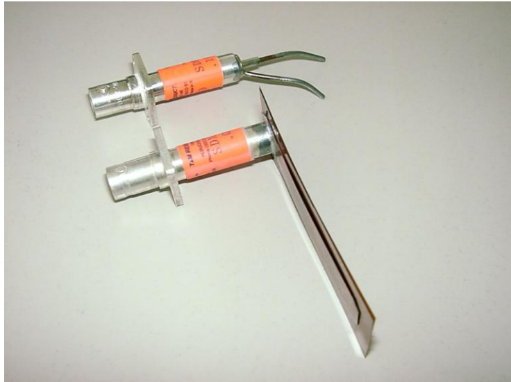
Picture 5: TTSDN shunt compared to standard catalogue SDN type
